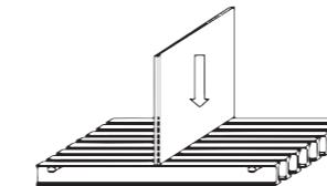
**Testing principle :** Measuring the deflection values of a specified testing sample with different concentrated line loads at different spans
