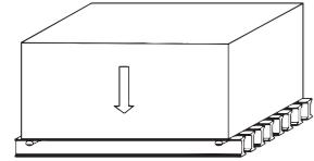
**Testing principle :** Measuring the deflection values of a specified testing sample with different uniform loads at different spans
